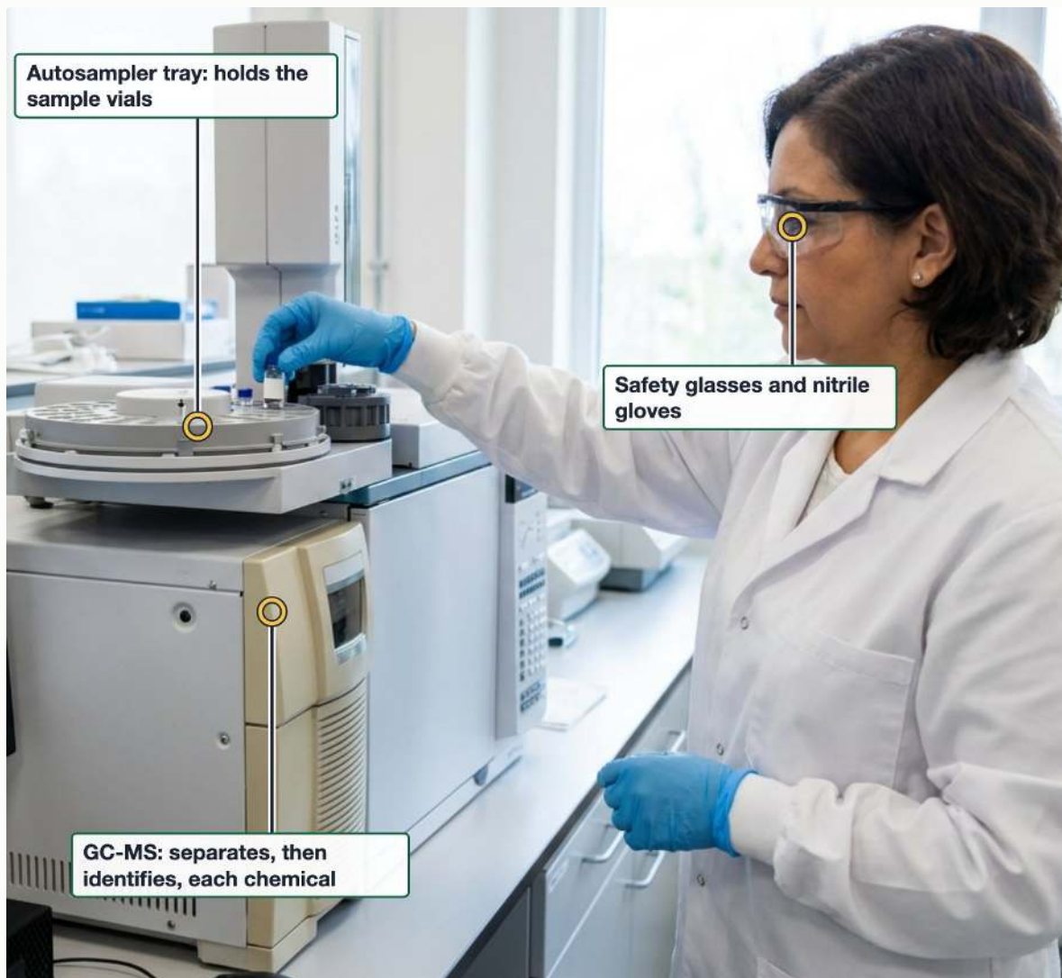
A forensic toxicology lab: a scientist loads a sample vial into a gas chromatograph with a mass spectrometer (GC-MS).
