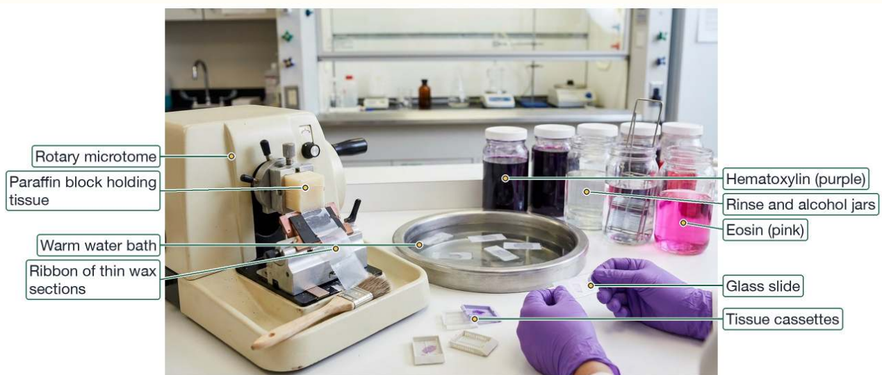
A histology bench: microtome, water bath, and the staining line from hematoxylin to eosin.
