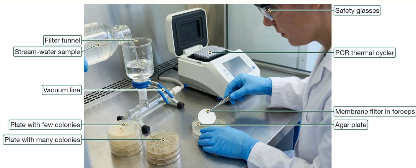
Environmental microbiology: stream water through a membrane filter, filters onto agar, colonies counted, genes checked by PCR.
