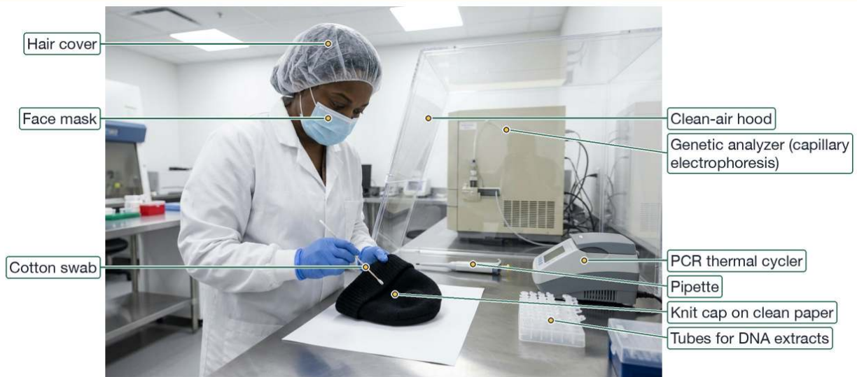
A forensic DNA lab: swab, extract, copy with PCR, then read each repeat length on a genetic analyzer.
