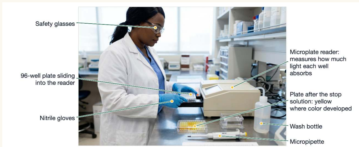
Figure S1b. A clinical ELISA: the 96-well plate goes into a microplate reader after the stop solution has turned developed wells yellow.
